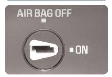
A key-activated switch in the glove box turns off the right-front passenger air
